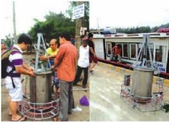
Experimental preparation of the electrical generator utilising sea wave energy on HQ1788 Ship
