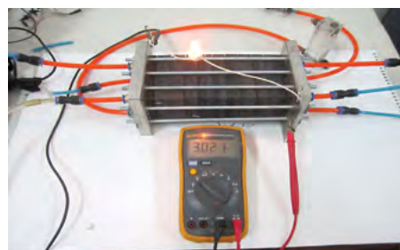
PEMFC stack, power ~ 20W
