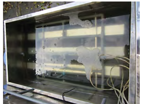
Oil contaminated wastewater treatment technology by using biofilm forming microorganism product in 300 litre/cycle module
