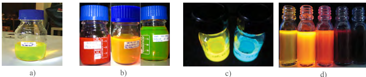
Photograph of CdSe/ZnS QDs in n-hexane (a); CdTe/CdS QDs in water (b); InP/ZnS QDs in n-hexane; and CuInS 2 /ZnS QDs in n-hexane (d).
